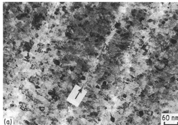
Figure 5 Cross-section of NiP/CoNiPt/overlayer in disk AMG1.
